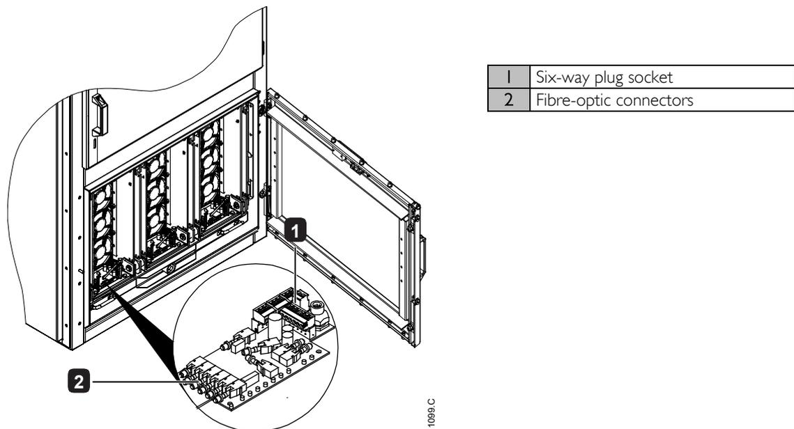
3. Locate the two fibre-optic cables, two-way connector plug and the six-way connector cable for the booster board.
