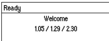
Software versions: Controller, control software, interface software
