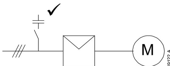
The soft starter must control the power factor correction capacitor contactor. Use the run output (terminals 33, 34 on the power interface board).
