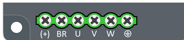
Fig. 4-7 LV-MD output (FS3) – Brake unit and Motor terminals
