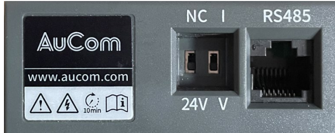
Fig. 4-2 LV-MD Control unit – Interfaces and LED indications
