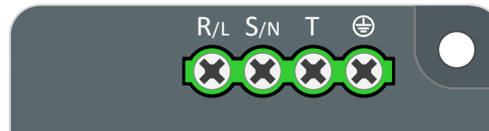
Fig. 4-5 LV-MD Input - Power supply terminals
