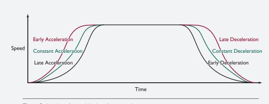
Figure 3: Acceleration and decleration control
