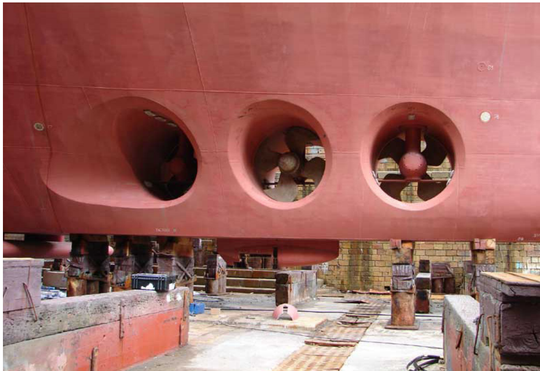
Application example: Soft starters are frequently selected for control of ship bow thrusters due to the large size of the motors relative to the generator.
